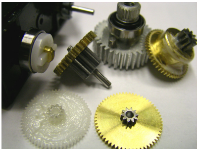
Fig. 11. The ground plastic gear (front-left) is replaced by the new metallic gear on the right. The servomotor then has a full set of metallic gear.
